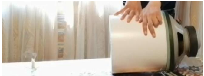
Figure 33. Flame suppression using the 400-watt speaker.
