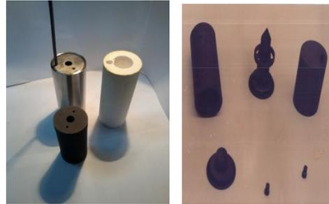
Fig. 1: Structures of silver point blackbody cavity
