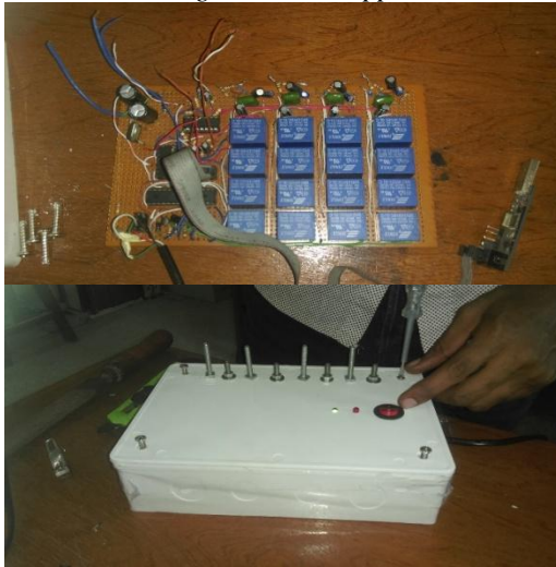
Figure 9: Constructed and Coupled Seismograph hardware showing all the components and units.
