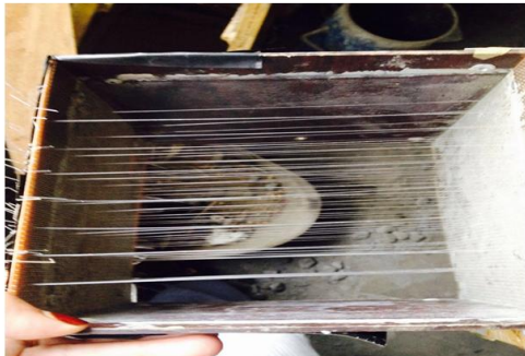
Fig 1 Inserting of optical fibers
