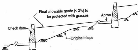
Fig. 5: Spacing Between Two Check Dams
