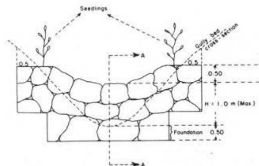
Fig. 3: A Loose Stone Check Dam. Source: FAO (1986)
