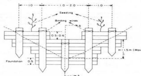
Fig. 2: Log Check Dam. Source: FAO (1986)
