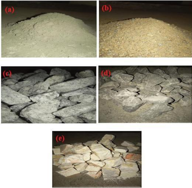
Fig. 1 (a) 53 grade Ramco cement, (b) fine aggregate, (c) granite, (d) basalt, and (e) marble.
