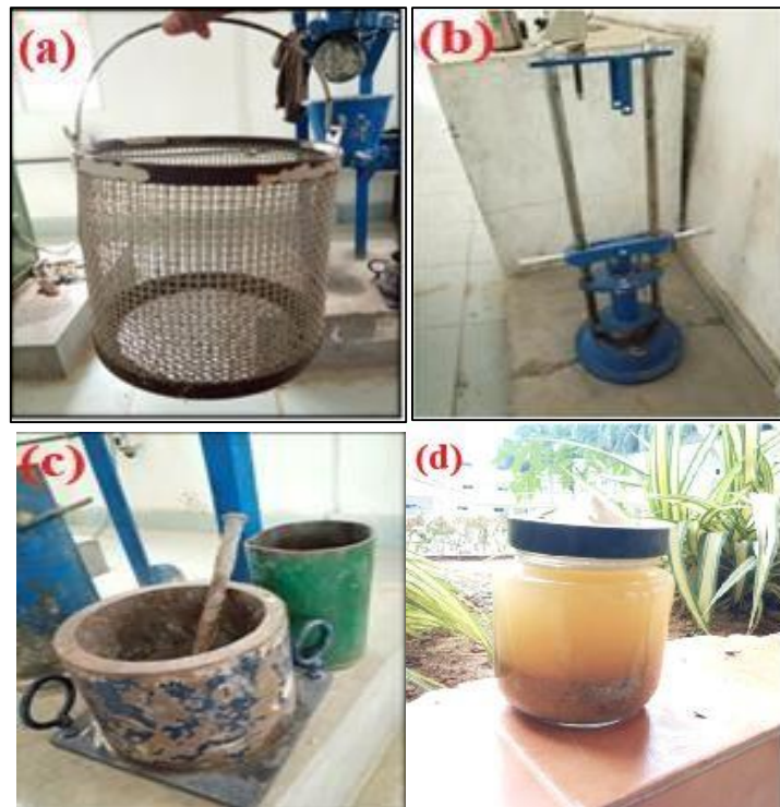
Fig. 2 (a) Wire basket used in specific gravity test, (b) Aggregate Impact value test setup, (c) Aggregate Crushing value setup, and (d) pycnometer.
