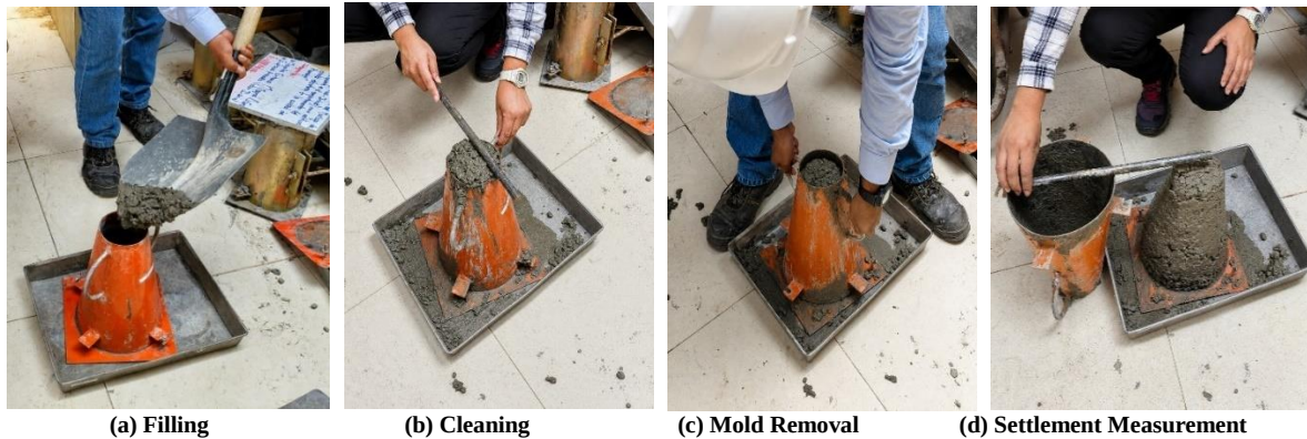
Fig. 2 Concrete Settlement Test Using the Abrams Cone Method.
