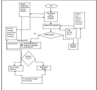
Figure 3: Flow Diagram Predictive-Reactive Technique
