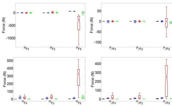
Fig. 11 Mean ( $\mu$ ) and Variance ( $\sigma$ ) of the force (F) and its differentials (F') for UCI dataset.
