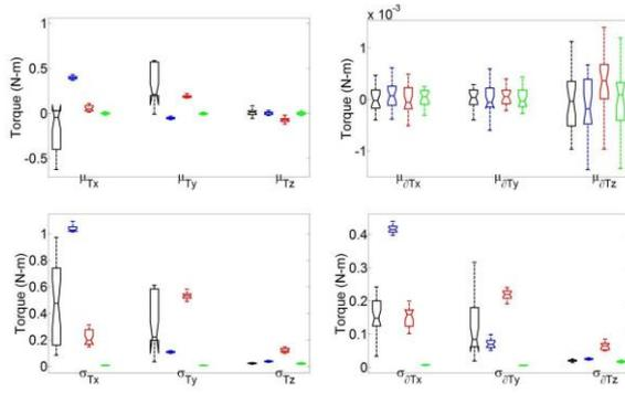
Fig. 8 Mean ( $\mu$ ) and Variance ( $\sigma$ ) of the torque (T) and its differentials (T') for Motoman MH-6 dataset.
