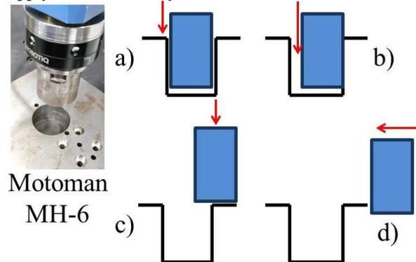
Fig. 1 (a) Normal, (b) jamming, (c) obstruction and (d) front collision.
