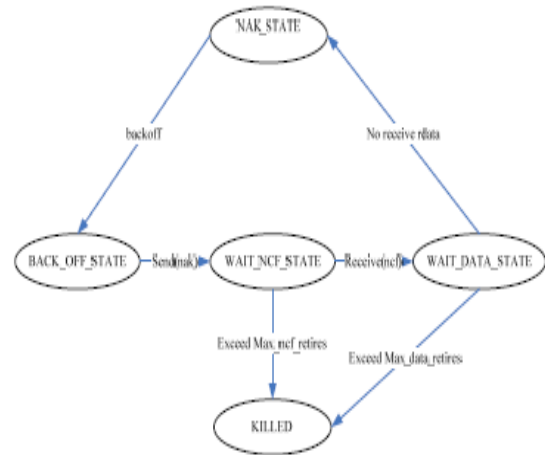
Fig. 2 State transition diagram of loss recovery scheme
