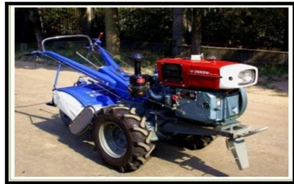
Fig.2 Power Tiller sprayer
