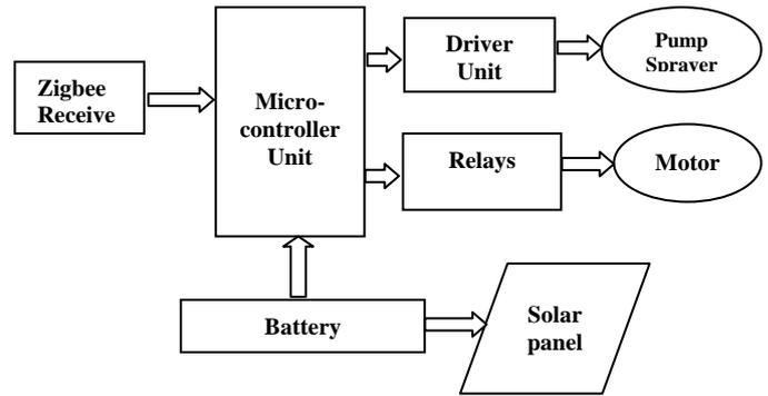
Fig.3.2 Block Diagram of Receiver
