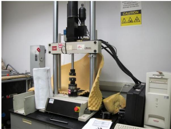
Figure 12: Universal Tensile Testing Machine
