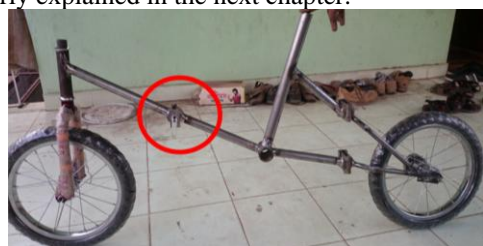
Fig 4.4: Area of Failure Highlighted
