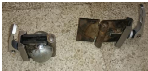
Fig 3.1: Fabricated hinge clamp system
