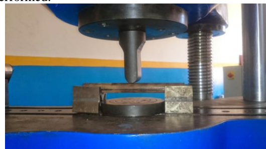
Fig 4.2: Specimen Setup on UTM for Bending Test
