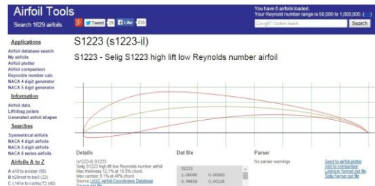
Figure 3: Shows The Profile of S1223Airfoil [3]
