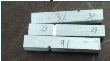
Fig 4: V-notch made to specimens for Izod test
