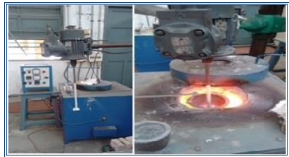
(a) Stir casting machine (b) Stirring using graphite impeller
