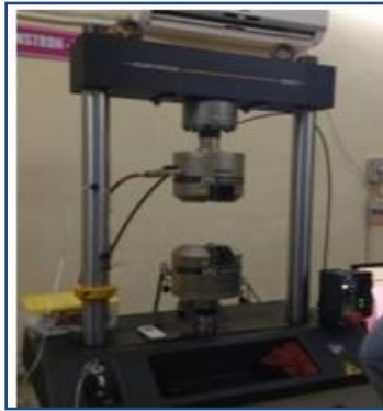
Fig 3: INSTRON Machine used for tensile test
