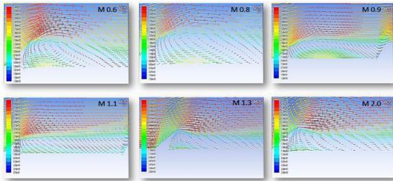
Figure 13 - Velocity vectors at wings of configuration 1 for all Mach numbers
