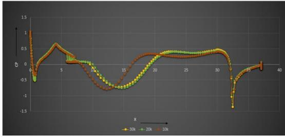
Figure 7 – The Co-efficient of pressure distribution over canard configuration for three different meshes at M 0.6
