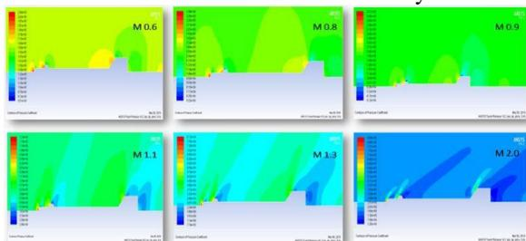
Figure 19 - Pressure contour comparison of configuration 2 for all Mach numbers
