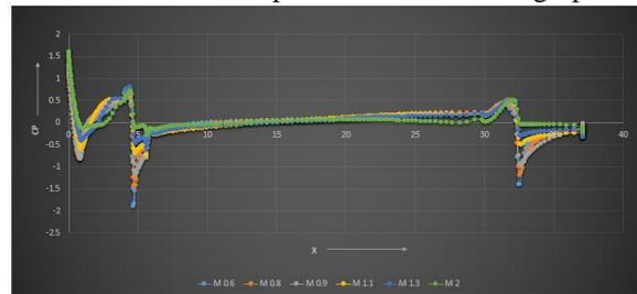
Figure 16 - Coefficient of pressure,  $C_p$  distribution over the configuration 2 for all the Mach numbers
