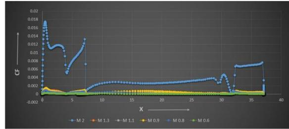
Figure 9 - Skin-friction coefficient, Cf distribution over the configuration 1 for all the Mach numbers
