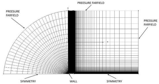
Figure 3 - Grid distribution and boundary conditions over canard controlled missile configuration
