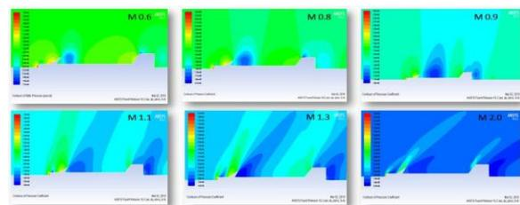
Figure 11 - Pressure contour comparison of configuration 1 for all Mach numbers
