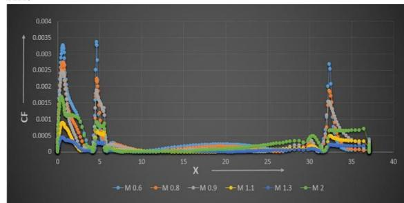
Figure 17 - Skin-friction coefficient,  $C_f$  distribution over the configuration 2 for all the Mach numbers
