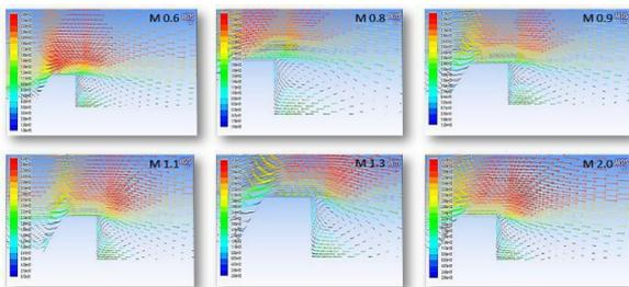
Figure 14 - Velocity vectors at fins of configuration 1 for all Mach numbers
