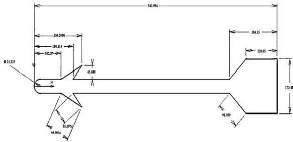
Figure 1 – Configuration 1 Geometric Details (All Dimensions are in mm)
