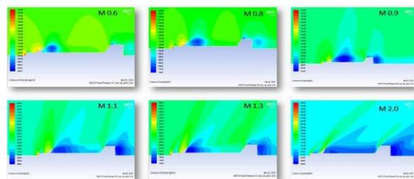
Figure 12 - Density contour comparison of configuration 1 for all Mach numbers
