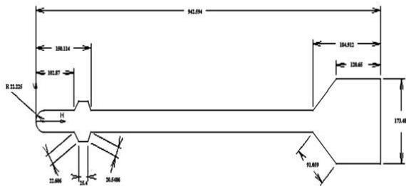
Figure 2 – Configuration 1 Geometric Details (All Dimensions are in mm)
