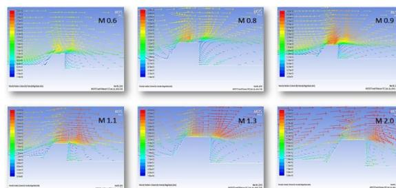
Figure 22 - Velocity vectors at fins of configuration 2 for all Mach numbers
