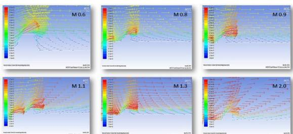
Figure 21 - Velocity vectors at wings of configuration 2 for all Mach numbers
