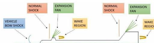
Figure 23 - The location of shock waves over Configuration 2
