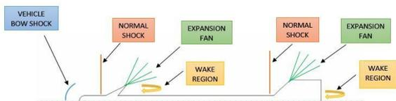
Figure 15 - The location of shock waves over configuration 1
