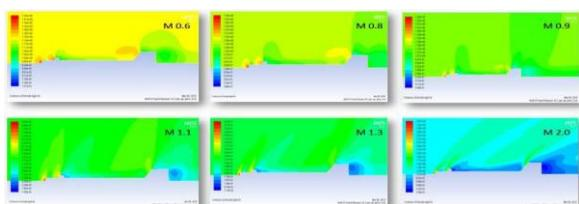
Figure 20 - Density contour comparison of configuration 2 for all Mach numbers
