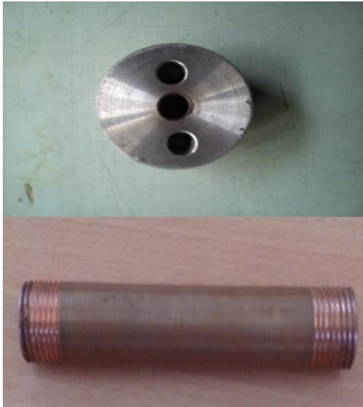
Figure 2. Fabrication of copper vortex tube parameters: (a) diameter orifices and (b) the hot end tube (c) the hot tube.
