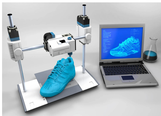
Fig. 3 Three-D printing or additive manufacturing of a shoe [15]
