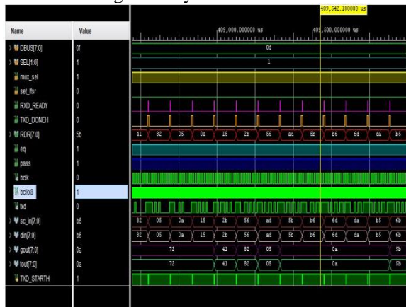
Fig 17: Simulation Results of the UART module
