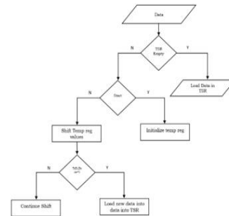
Fig 15: Flow chart of the UART Transmitter
