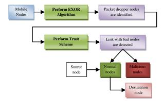
Fig.2. Block diagram of proposed algorithm
