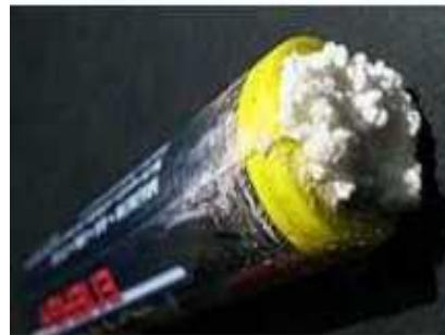
Fig1. A Leaking Electrochemical Battery.
