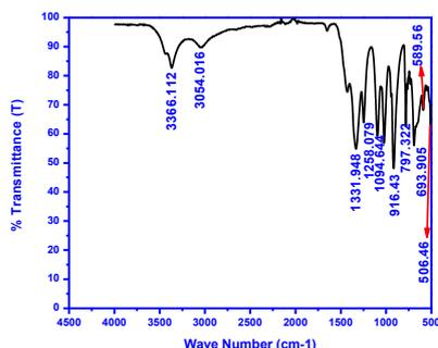
Figure (3). FTIR Spectrum of LTKB5 crystal
