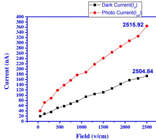
Figure (5). Field dependent photoconductivity of LTKB5 crystal the orthorhombic structure of the crystal. The SHG efficiency confirms an appreciable NLO property.
