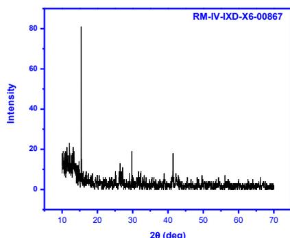
Figure (2). Powder XRD pattern of LTKB5 crystal
