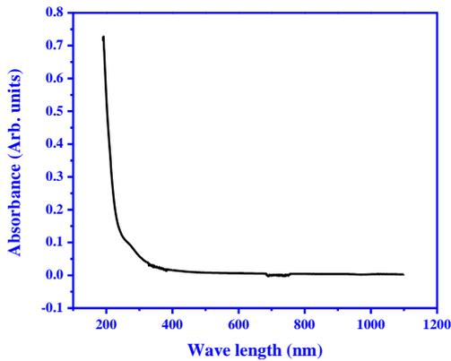
Figure (4). Absorption spectrum of LTKB5 crystal
