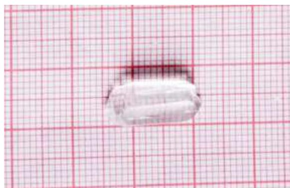
Figure (1). Photograph of L-Threonine Doped KB5 Crystal
