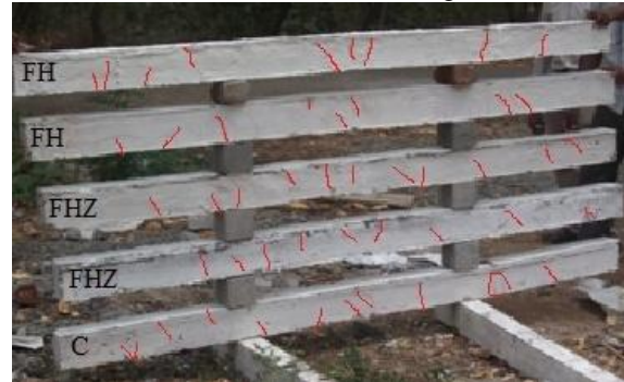
Fig Failure pattern for all the beams
