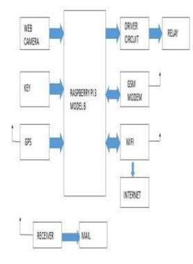
Fig.1.Block Diagram of smart security system for two wheelers
