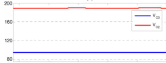
Fig 9: (B) show the voltage across the DVCM stage capacitors vc3 & vc2
