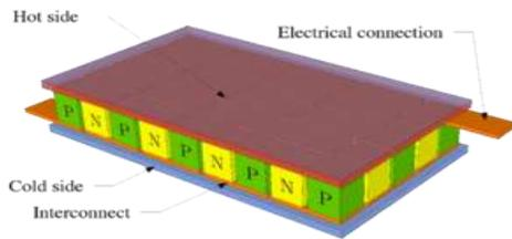
A single station thermoelectric defervescent will typically show a maximum mixture distinction of 70 c between is passionate and cold sides. The more heated moved using a thermoelectric jail, the less competent if becomes, for the thermoelectric jail needs to diffuse both the vehemence being moved and the heated it cause itself from its own command consumption, the amount of heat that can be wrapped is relative to the passable and measure
