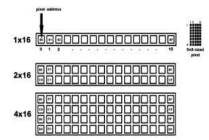
Above figure shows that each LCD have its own pixel rows and columns like  $1 \times 16$  has weak unpracticed and sixteen columns i.e. 16 pixel and each pixel adjust is of  $5 \times 8$  as shown but we can see only  $5 \times 7$  reason last unwrought is habit by cursor. Each character is descry according to these pixels size.
