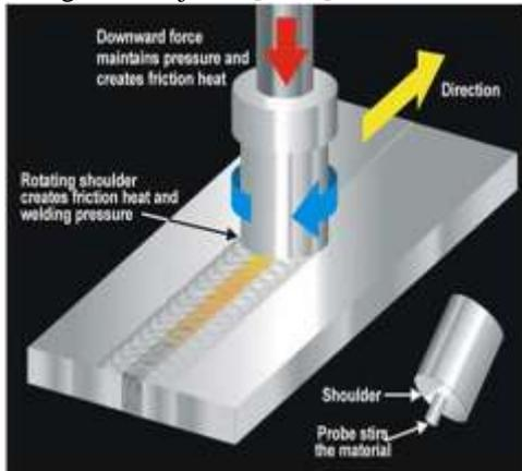
Figure-2: FSW Process principle [6]
