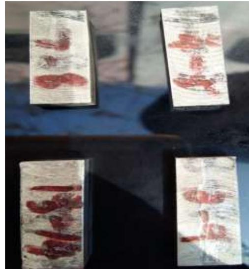
Figure-5. Specimen before wear test
