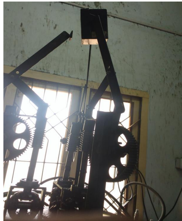
Fig 4; when 2 fingers blocked with object and remaining 1 finger continue to move
