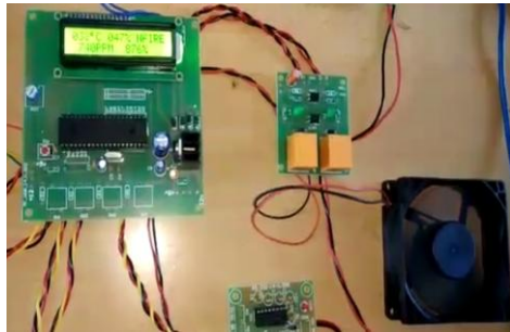
Fig. 6(a). Exhaust fan is switched ON
