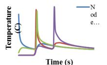
Fig. 8:Temperature histories at point A, B, C and D for welding sequence A
