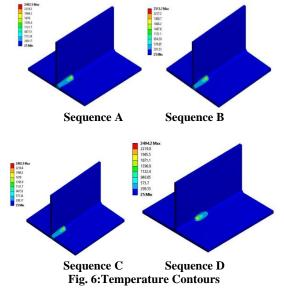
It is observed that temperature distributions around the source are typical of the fusion zone (FZ) and the heat affected zone (HAZ). It is also noticed that the heat source preheats a small region of weld plate ahead of the moving heat source. The peak temperature at the center of fusion zone is in proportion to the heat input. The heat generated by the moving heat source along the weld is gradually propagated towards all directions in the plate through conduction, convection and radiation.
