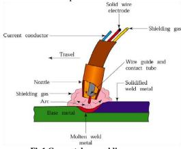
Fig1.Gas metal arc welding process
