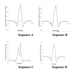
Fig. 12 : Transverse residual stress distribution for welding sequences
