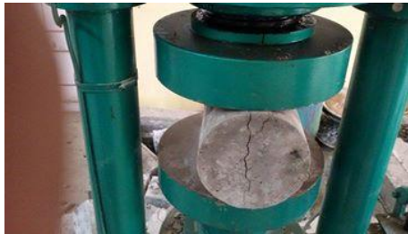
Figure 8.3: Picture shows the Split tensile strength
