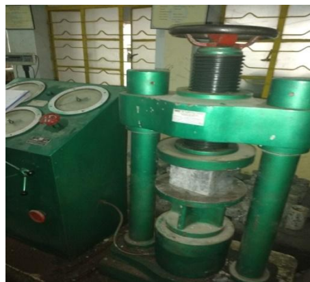
Figure 8.1: Picture showing the compressive testing for cubes
