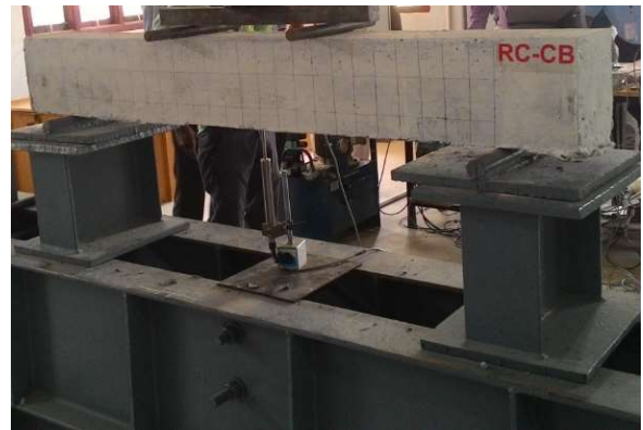
Fig 4: Beam subjected to two point loading on loading frame
