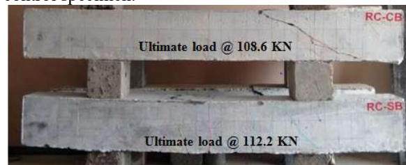
Fig 9: crack pattern of RC-SB & RC-CB
