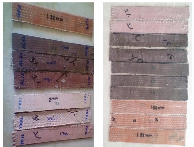
Fig 3 : GFRP composite polyester with and without Al and TiO 2
