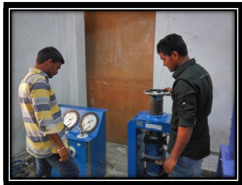
Fig 5: Finding crushing value of the aggregates
