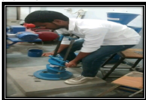
Fig 6: Finding Impact value of the aggregates
