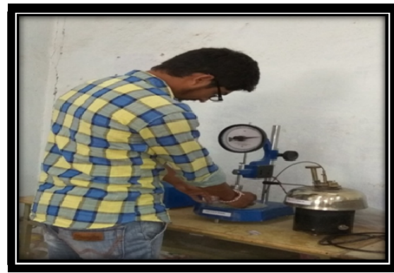
Fig 7: Finding penetration value of the bitumen
