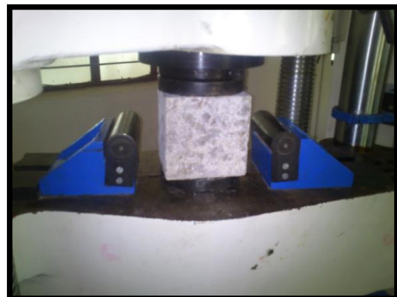
Figure - 5 Compressive test setup
