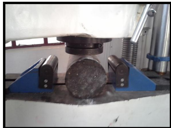
Figure - 6 split tensile test setup
