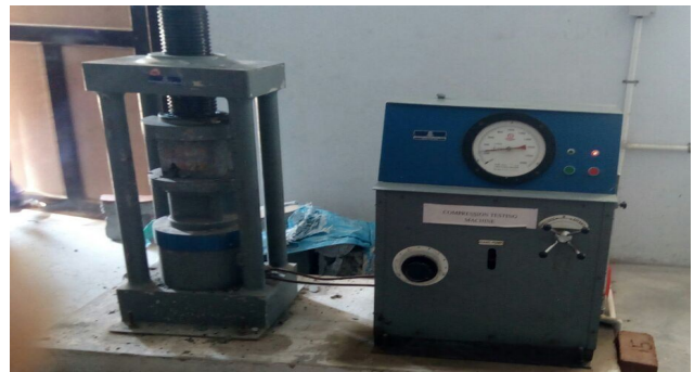
Fig .5 Compression Test For Cube
