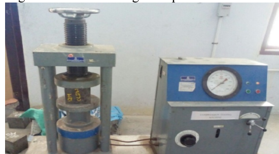
Fig .4 Compression test on geopolymer concrete
