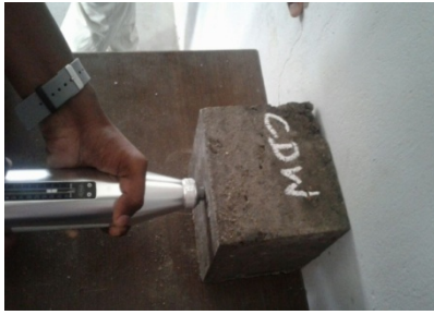
Fig.5 Rebound Hammer Test on geopolymer concrete
