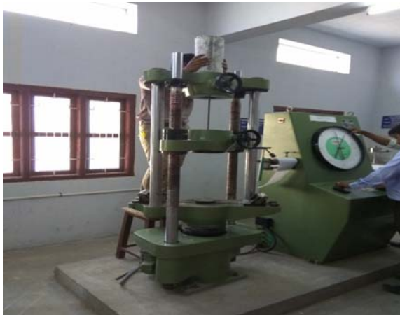
Fig 4- Pullout strength Test
