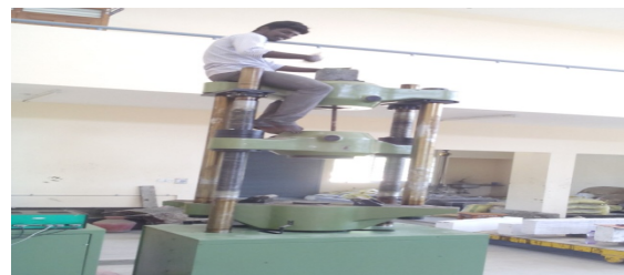
Fig 2 : BOND STRENGTH TEST
