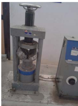
Fig 2 Strength Test For Cylinder
