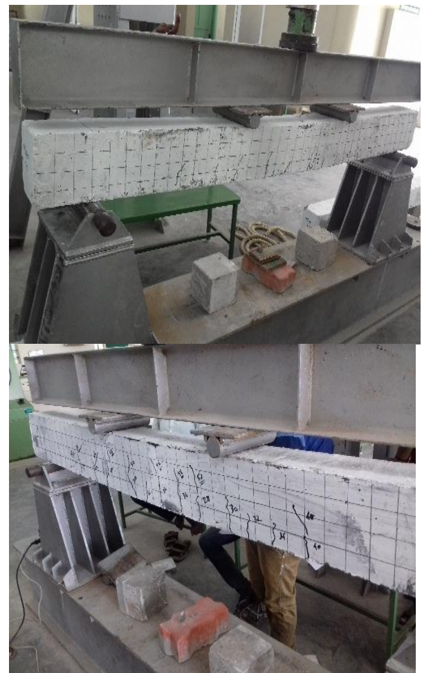
Figure 9: Beam Test and Crack Pattern
