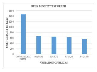
Figure:4.1. graph for bulk density test results
