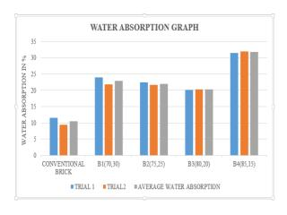
Figure 4.3 Graph of Water Absorption test
