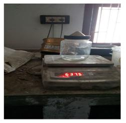
Figure: 3.1. specific gravity test
