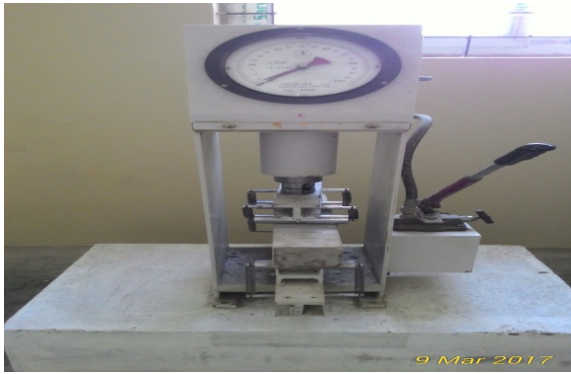
Fig. 9. Flexure test- Vertical joint
