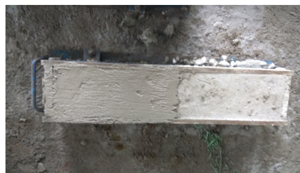
Fig. 4. Concrete casted fully/partially.
