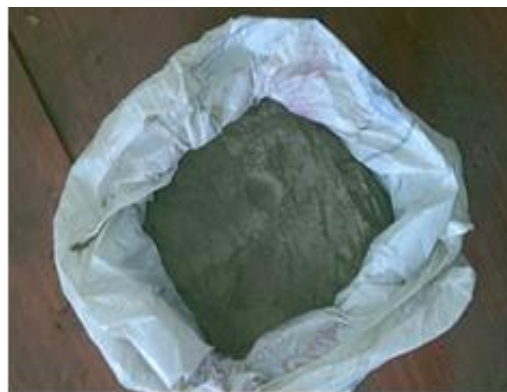
Fig 1.2 Fly ash (Class F)
