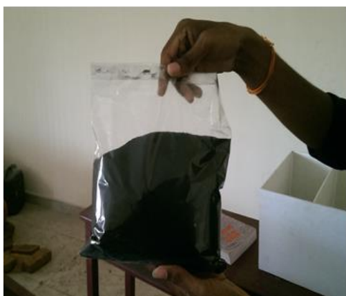
Fig 1.1 Crumb rubber (30 mesh)
