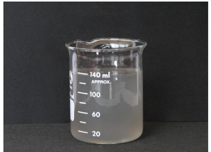
**Figure 5 Sodium silicate solution**
