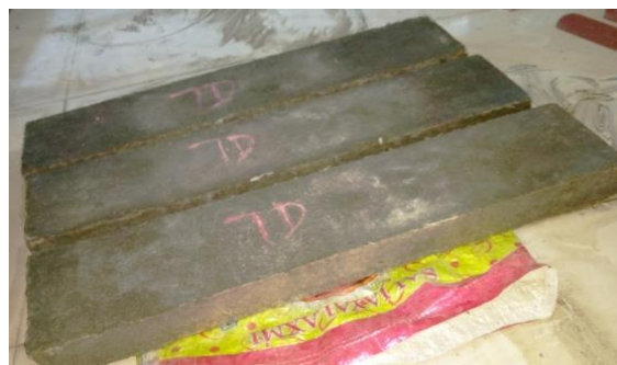
Fig.3. ECC concrete slab with 60mm thickness after demoulding.
