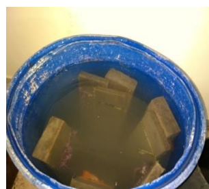
Fig.4. Curing of slabs.
