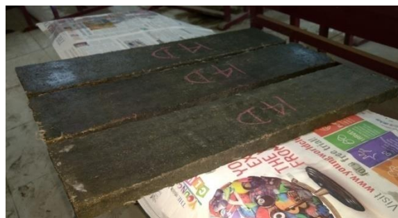
Fig.3.1. ECC concrete slab with 30mm thickness after demoulding.
