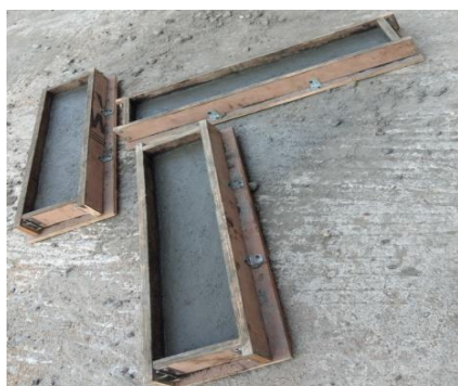
Fig.2.1. Casting of ECC concrete in slab.
