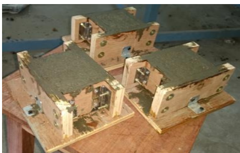
Fig.2. Casting of ECC concrete in cube.
