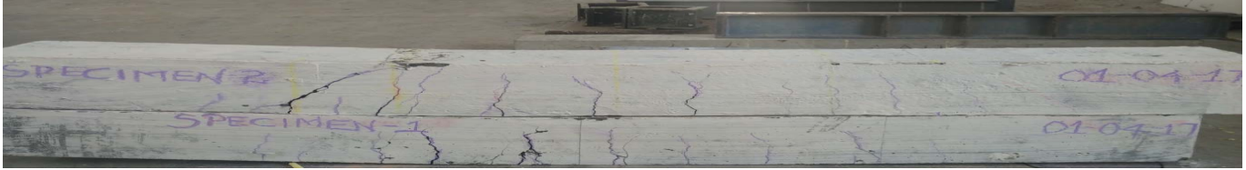
Figure 3: Comparison of beams under flexure and shear mode of failure
