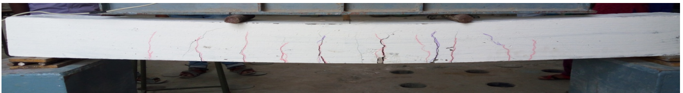
Figure 1: Performance of beam (1) under flexure mode
