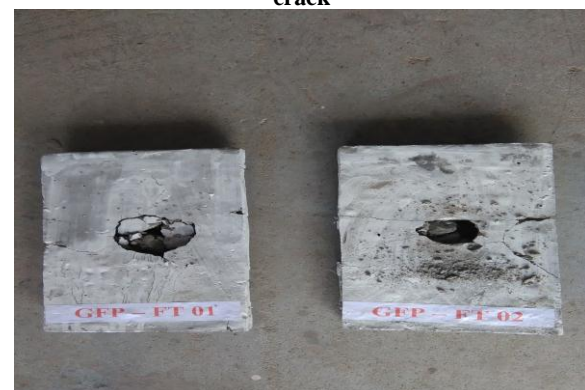
Figure 7. Geopolymer Ferrocement Flat Panels at failure
