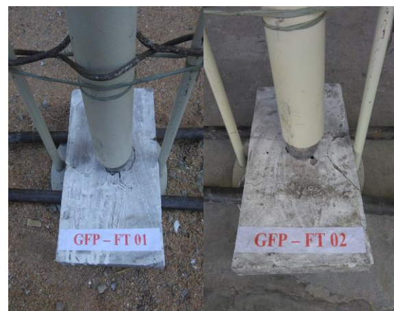
Figure 6. Geopolymer Ferrocement Flat Panels at First crack
