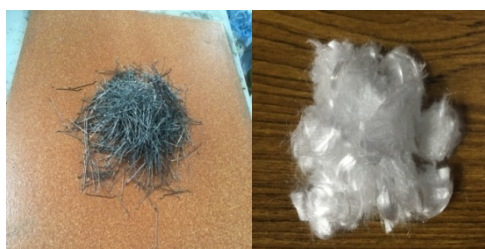
Figure 1 Steel and Polypropylene Fibre
